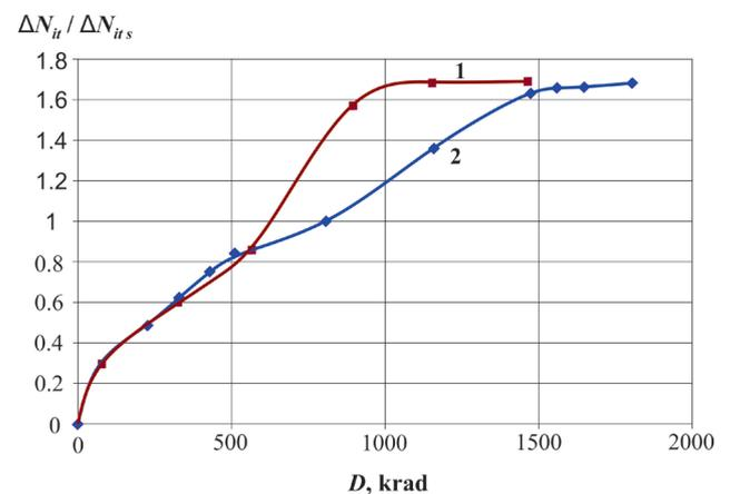
the performance of MOSFETs in the fields of low-intensity radiation from outer space. As shown in Fig. 2, surface defect formation at the first “dose” stage may not lead to failure. Then the failure will occur in the second stage, but after a longer period.
